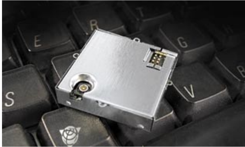
Lassen SQ GPS receiver with metal shield
