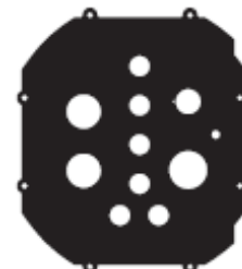
VT-EC08a · 6x 0.250" circular · 1x 0.250"x0.450" D-Hole · 1x 0.125"x0.225" D-Hole with 0.95" Locking Hole
