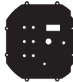
VT-EC09a · 4x 0.50" 0.465" D-Hole · 2x 0.540"x0.563" D-Hole · 2x 0.895"x0.824" D-Hole · 1x 0.940"x1.01" D-Hole · 1x MS3404D10SL-3P Circular with 0.095" Locking Hole
