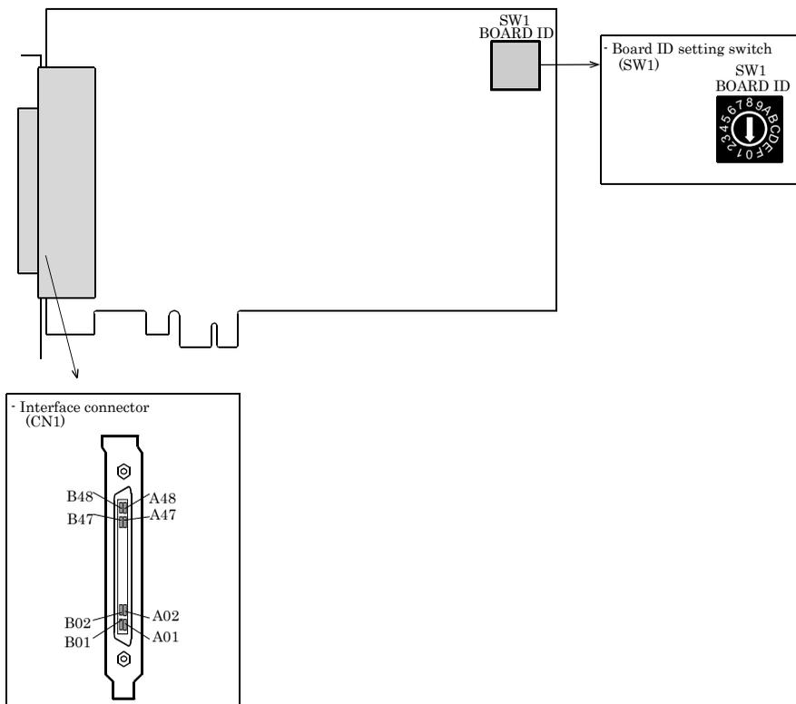
**Figure 2.2. Component Locations < DIO-3232RL-PE >**
