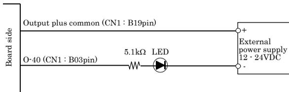
**Figure 3.10.** An Example to use Output O-40 < DIO-3232RL-PE >
