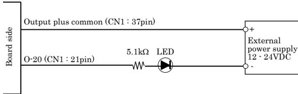
**Figure 3.9.** An Example to use Output O-20 < DIO-1616RL-PE >
