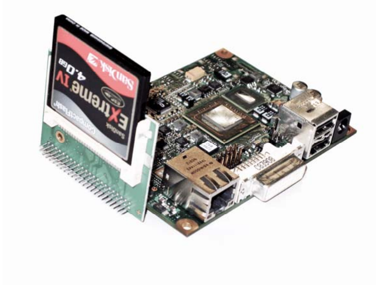
KONTRON CF card adapter (CF-CARD-adapt-MOPS, part number 40404)
