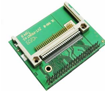
KONTRON CF card adapter (CF-CARD-adapt-MOPS, part number 40404)
