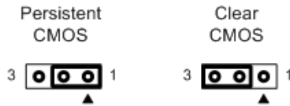
Figure 9: Jumper Block JBAT1 Settings
